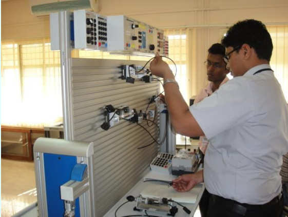
Fluid power circuits
